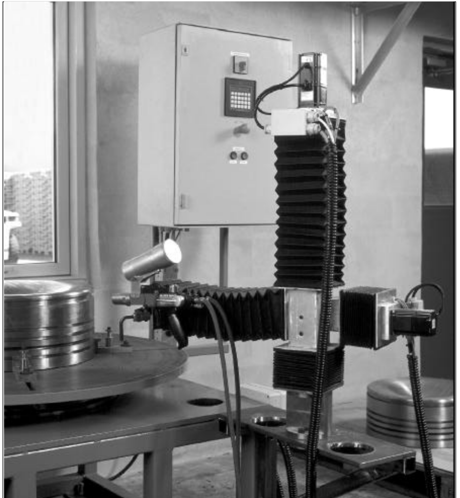
Experimental set-up for powder flame spraying the grooves of a 50cm piston head.
