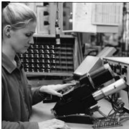
Workplace for calibration of pressostats/thermostats.
